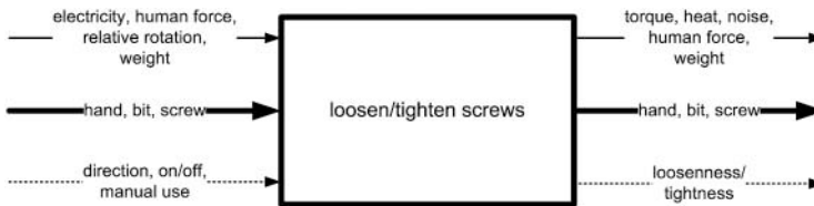
Figure 3. A functional description of the power screwdriver (from Stone and Wood 2000).
