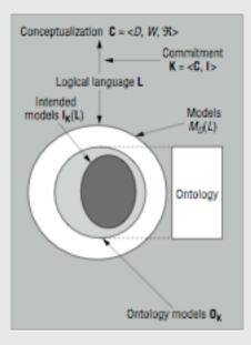
The relationship between an ontology and a conceptualization. Given a logical language L that implicitly commits to a conceptualization C, an ontology's purpose is to capture the models of L that are compatible with C. These models are called the intended models.
