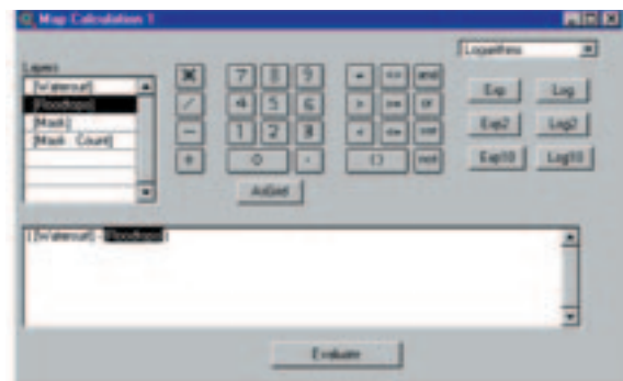
FIGURE 14.4 Calculating the water depth in the floodplain
