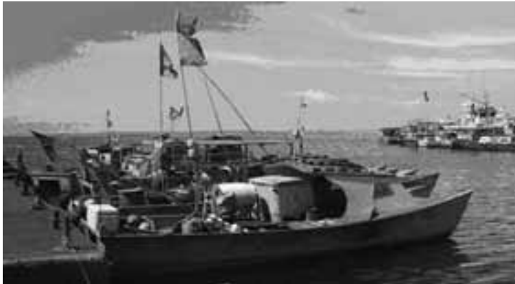
Small alias with an icebox ready to locate within the cabin. Space is limited but the catch can now be cooled immediately on landing aboard the vessel
